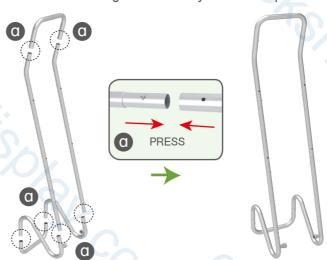
STEP 03 To install the cross bar according to labellings
