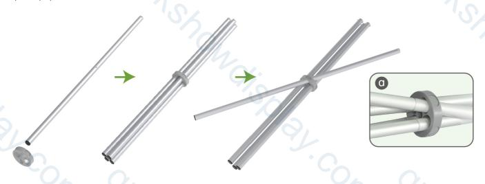
Press poles' knobs to clip into countertop's slot.
